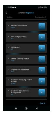
For example, let's say that the selected module is the Digital diesel electronics (DDE). This module should be pressed.
