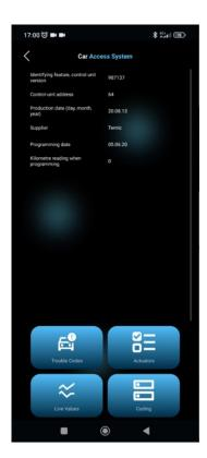
After that the "Coding" button on the display should be pressed and the opportunity to select from the available "fast coding" options should be provided.
