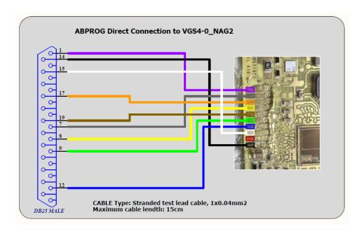
Here is where you have to cup open the plastic cover of the TCU in order to get access to the PCB for ABProg connection.
