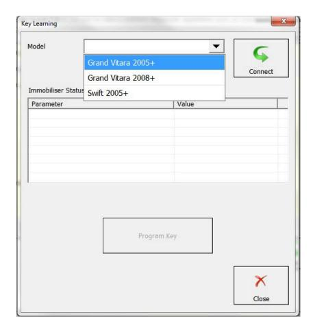
After selecting the vehicle the user should press connect and the connection to the vehicle will be established.
