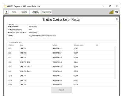
Once you have selected the unit and the appropriate version to start the process, you will see the screen with instructions and a larg "START" button. To continue, you need to press and hold the START button. The software works as a guided function and is very intuitive to follow. If you are missing the required license you will get a message as in the second screenshot of this page.
