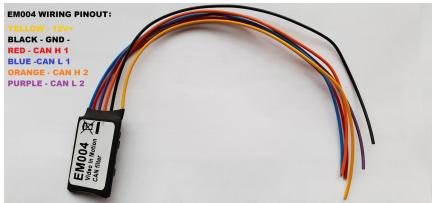
The Comfort CANBUS needs to be interrupted and the EM004 needs to be soldered to the CAN H and CAN L. You can easily tell them apart from the rest of the cables when you take the head unit out. The cables for the comfort CAN are
