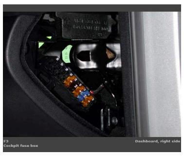
W164 passenger fuse box. EZS fuse is socket 14
