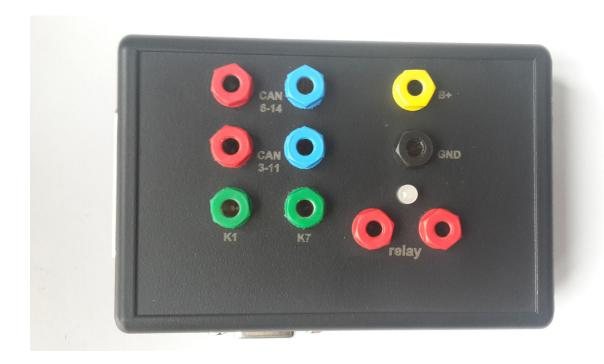
1st two ports (Red and Blue) are for CAN HI and CAN LOW 6-14, the 2nd ports below them are for CAN HI and CAN LOW 3-11. These ports are mainly used when virginizing and adapting Mercedes TCUs and ECUs when using MN026.
