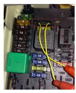
When working on a W204 car for all keys lost for example you can open the front SAM module on the driver side and see fuse number "27" - disconnect it, connect your ABRITES FUSE RELAY CONNECTOR and plug your relay and proceed to start the All keys lost procedure. Make sure that the ZN036 is in the EZS and that it is in the ignition "ON" position.
