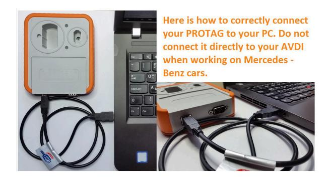
Depending on the situation you can use different methods of password extraction. If you have a working key you can use your working key with your PROTAG programmer in order to easily extract the password. When you use this method you need to put the key in the EZS and in the PROTAG in a sequence. The software will give you the needed instructions.
