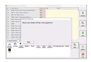
5. At this step you have to place each of the existing car keys(if available) in your PROTAG programmer prior to key programming of the new keys, or place directly a new Abrites TA54/TA56/TA57 JLR key if it is an All Keys Lost situation.
