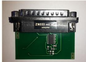
Using the ZN033 NEC MCU Adapter, you will be able to solder NEC processors used in Mercedes keys, read them and make them virgin. The supported versions are V57 and some V51.
