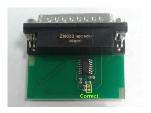
Once the NEC MCU is soldered to the ZN033 Nec MCU Adapter, the ZN033 has to be connected to ZN045 ABPROG. The ABPROG can be directly connected to AVDI as shown in the picture below:
