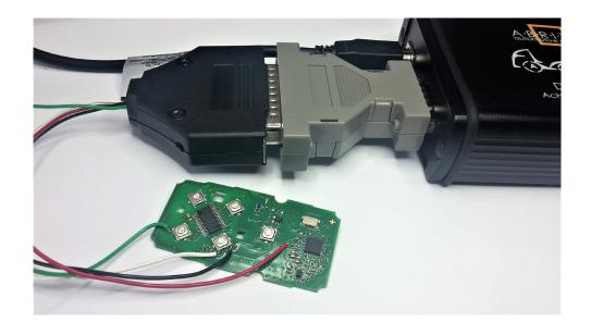
Once the cables of the ABPROG Adapter are soldered to the PCB, the ABPROG software can be started:
